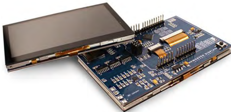
Figure 7. The Newhaven Displays NHD-4.3CTP-N, daylight readable and touch-responsive.
