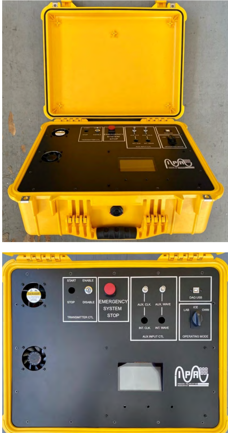
Figure 15. Marine IP prototype enclosure with custom internal and external panels.
