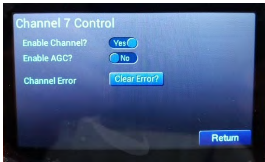
Figure 10. Example selection screen for channel control. Colors selected to be user friendly for color deficient operators.
