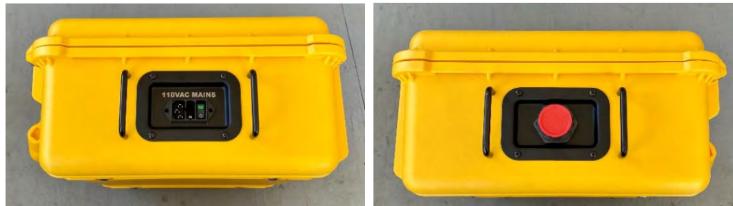
Figure 2. Marine IP enclosure. (Left) The left side of the box, AC power, mains input. (Right) The right side of the box, water-resistant ingress port for the Marine IP cable connector.
